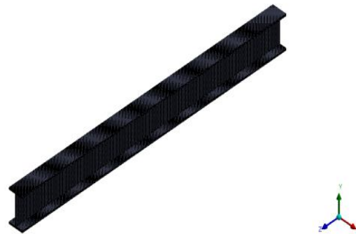
Fig.14.Mesh Model of I-Section Beam
