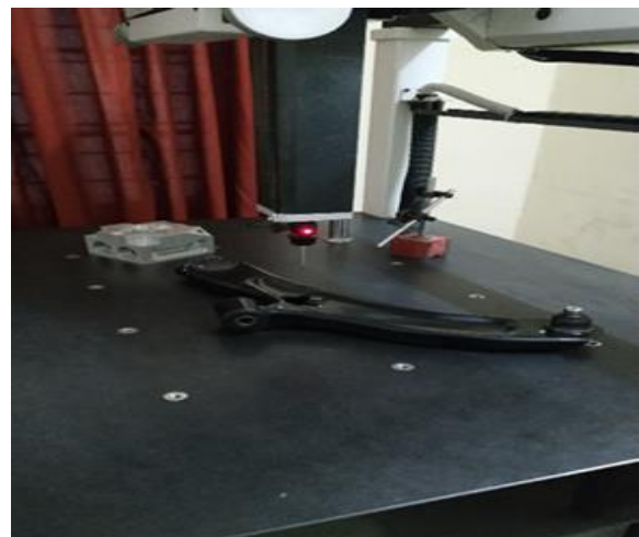
Fig. 3 CMM of Lower Control Arm
