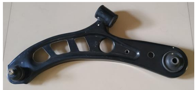
Fig. 14 Optimized Lower Control Arm
