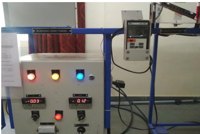
Fig. 10 Wind Tunnel Setup with Annemometer
