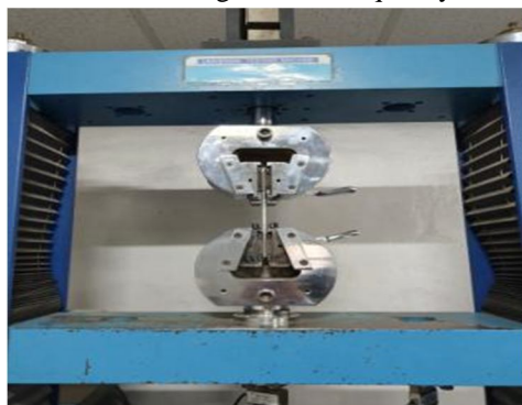
Fig. 1. Tensile strength testing (ASTM D638-2014)
