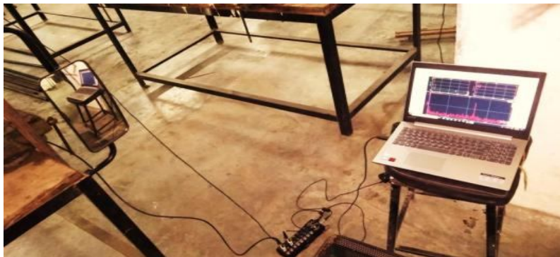
Fig no. 29 Experimental setup for Modal Analysis for Iteration 3 Design.
