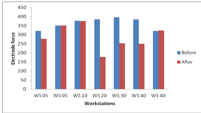
Graph 1 Weld Force Comparison for One-T
