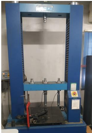
Fig. 15 Testing of LCA under UTM
