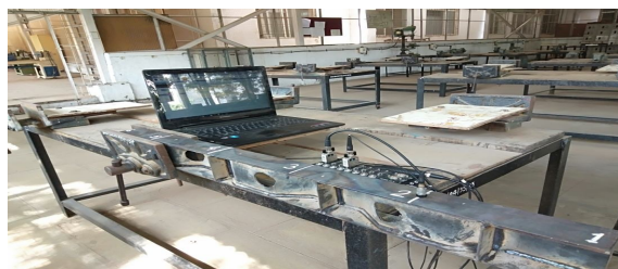
Fig.25. Experimental Testing of Modified I-section Beam
