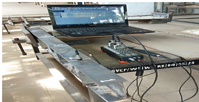
Fig.26. Experimental Testing of Trapezoidal corrugated web Beam
