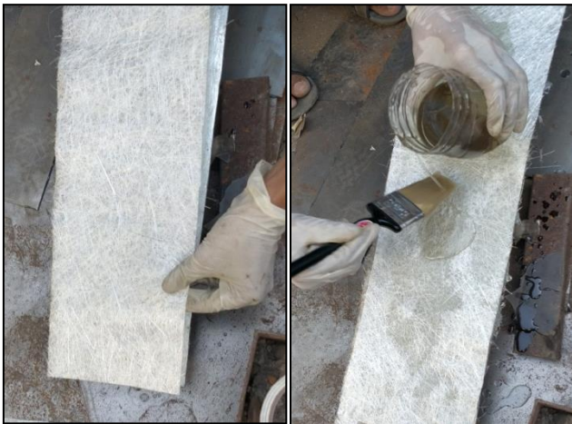
Fig. 12: Manufacturing process of composite leaf spring
