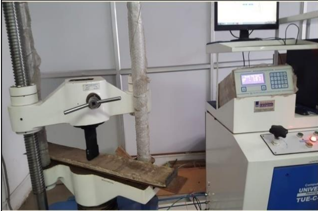
Fig. 13: 3-point bending test on UTM
