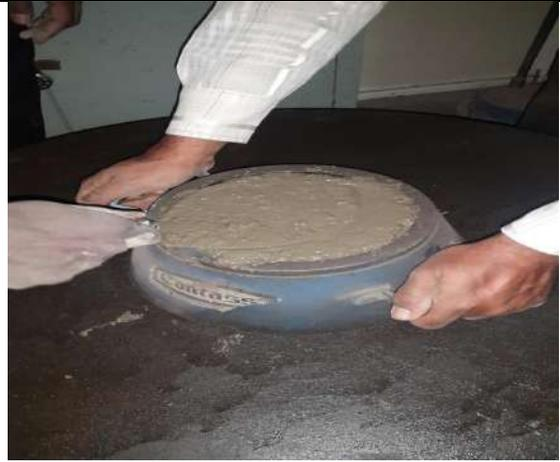
Slump Cone & Flow Table test for checking workability
